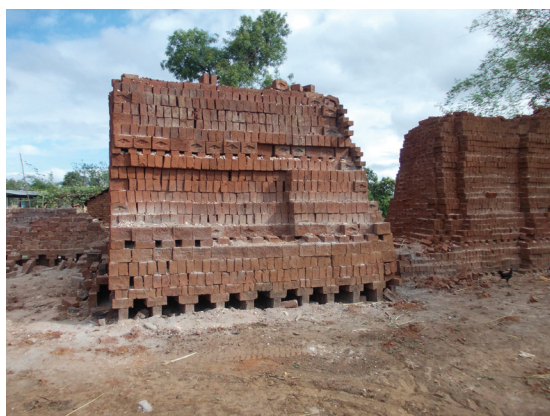
A small-scale clamp. Small-scale clamps produce between 10,000 to 25,000 bricks
