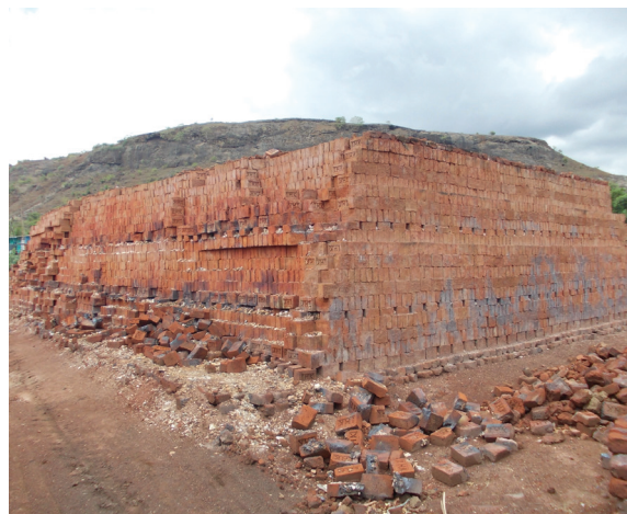
A typical clamp in the area producing around 3–4 lakh bricks per batch
